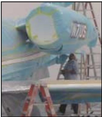
When the base color has been applied, the computer-controlled booth goes into Dry Mode at ambient temperature and humidity for two or three hours to let the paint “breathe.” Then it switches to Dry Mode 2 and the temperature goes up to 110 degrees for six hours, after which it shuts down automatically.
