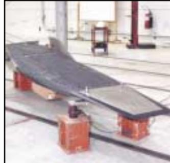
During ground testing, NASA's 2,800-pound, 12-foot X-43A scramjet resembles a large, black sled.
