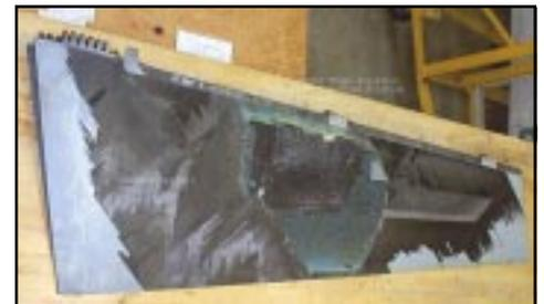
**Gone with the wind** -- An F/A-18 rudder shows extensive damage after honeycomb core rot caused an inflight failure.
