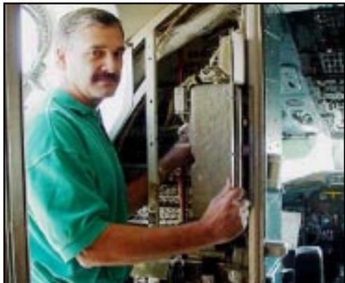
**No arcs, no sparks** -- Chuck Saye, an engineer with the Naval Air System Command's C-9 engineering team, monitors a C-9 circuit breaker panel during recent ground testing of the arc fault circuit breaker.
