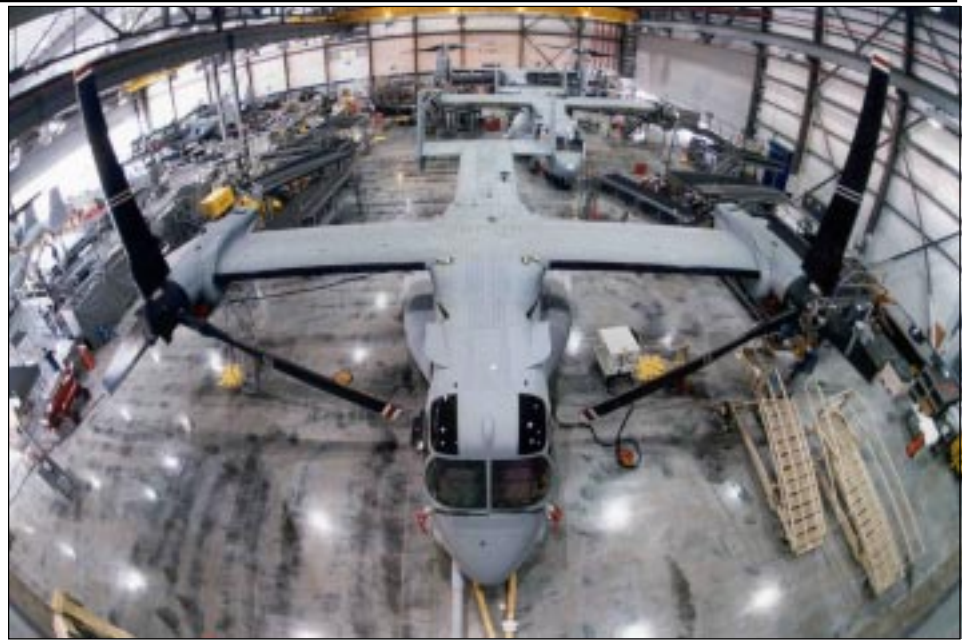
Final assembly of each MV-22 using lean manufacturing methods saves time, space and money.
