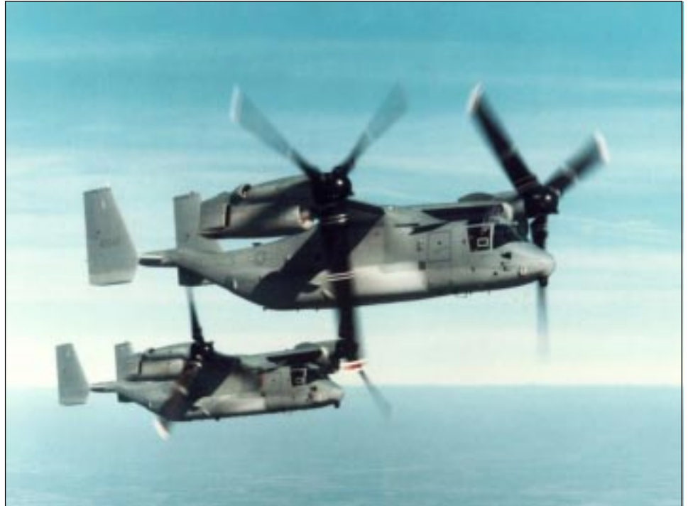
The OPEVAL Report revealed that the V-22 is overwhelmingly superior to the aging CH-46E, including twice the speed, five times the range and three times the payload capacity.
