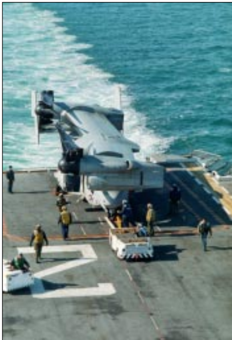
The V-22 will undergo additional evaluation of its Blade Fold Wing Stow system Nov. 15.
