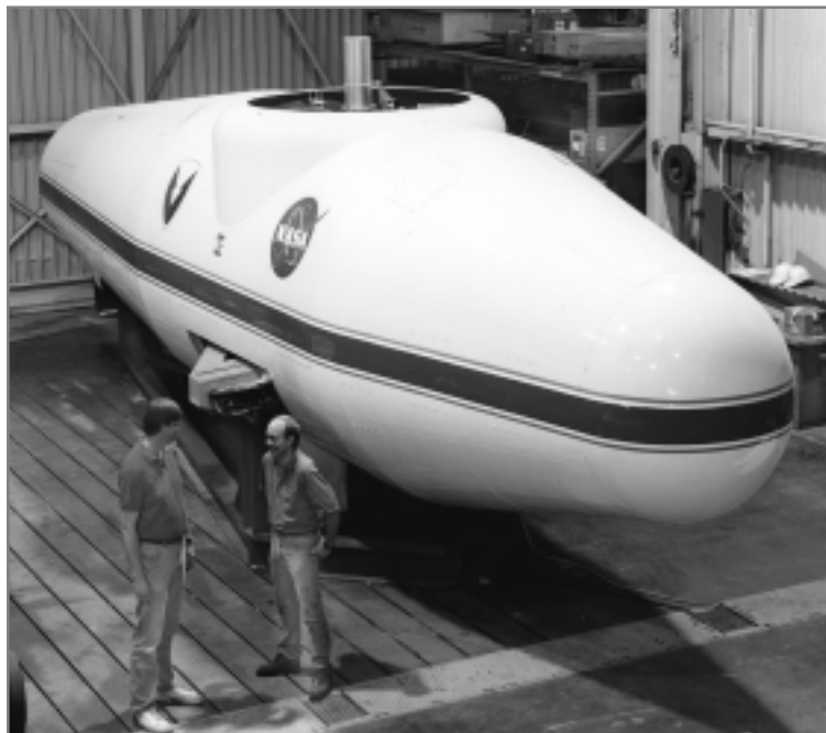
The LRTA (shown here in Building 246) is a wind tunnel test stand designed for testing moderate-to-large helicopter and tiltrotors.
