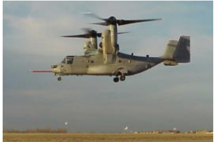
Number 7 at Bell's Arlington Plant 6. The terrain-following radar and flight test boom are visible off the nose. Photo by Jim Jagodzinski, Bell Helicopter.
